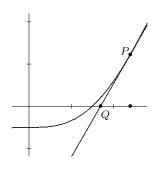
775. Use Newton's Method to solve  $x - \sin x = 0.5$ . This means finding the unique zero of the function defined by  $f(x) = x - \sin x - 0.5$ , part of whose graph is shown above. As suggested by the figure, start with the guess  $x_0 = 2.4$ , and stop when you get to  $x_4$ , which will be accurate to seven decimal places.
